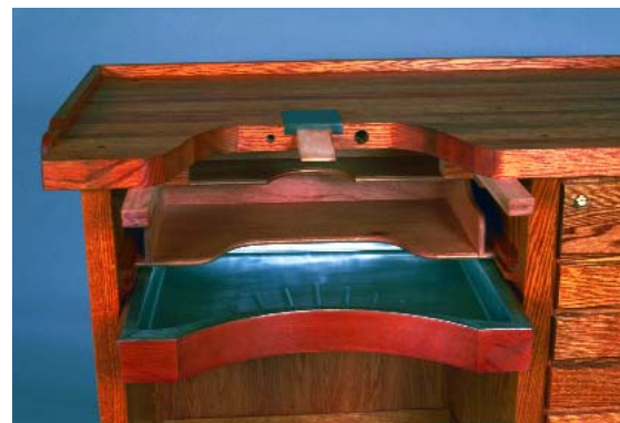
Detail of locking drawer, layout board, catch pan and bur tray.
