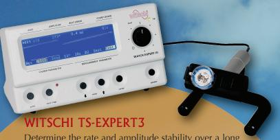
Determine the rate and amplitude stability over a long period of time, viewing deviation, beat error and noise, plus amplitude. Automatically select all common beat numbers or manually select 3,600-43,200 beats (6Hz) per hour. Print the rate, beat error, and amplitude.
