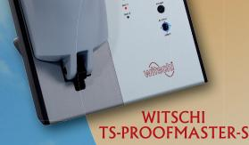
Pressurize from .2 to 10 BAR and vacuum to -.7 BAR to detect small and large leaks. If leak is small, pressure will remain inside the watch to show air bubbles under water.
